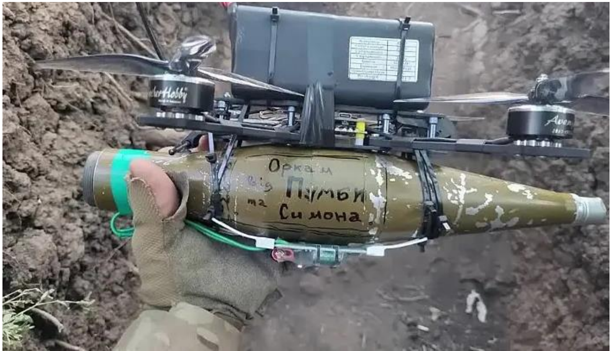
Fig. 4 – Ukrainian FPV-kamikaze UCAV with an attached charge from PATGL 13 .
