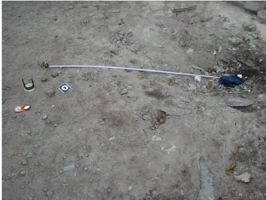
Fig. 14 – Determining the direction of an artillery projectile trajectory.
