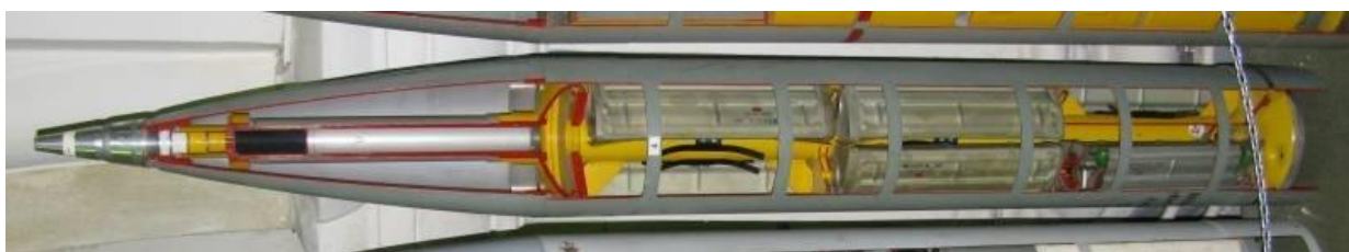
Fig. 1 - Dummy 9M27K3 projectile with anti-personnel mines.
