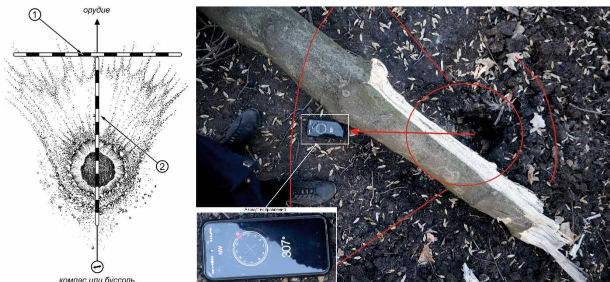
Fig. 48 – Determination of the shelling direction by the controlled fragmentation method.
