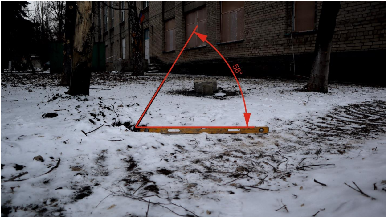
Fig. 49 – Determining the angle of impact with a horizontal surface at the site of shell hit 2 of December 19, 2022
