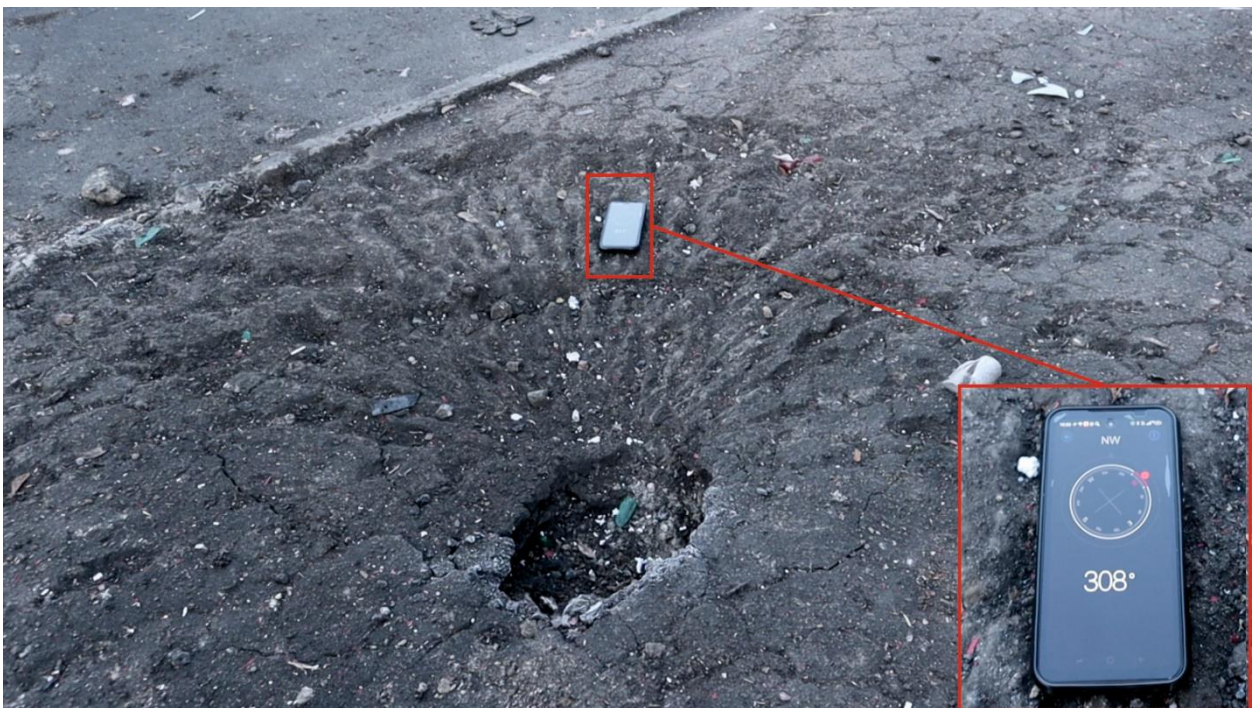
Fig50 – Azimuth determination at the site of shell hit 7 of December 19, 2022
