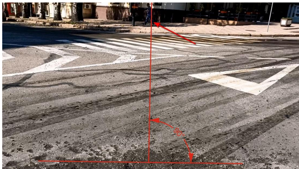
Fig. 22 – Determination of the intersection of the azimuth along which the projectile moved with the wall of the building at 16, Pushkina Blvd.
