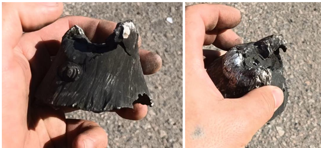
Fig. 14 – Detonating fuze found at the site of shell hit 6.
