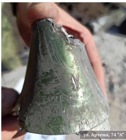
Fig. 15 – A NATO-standard PD.M739A1 fuze found by the JCCC representatives.
