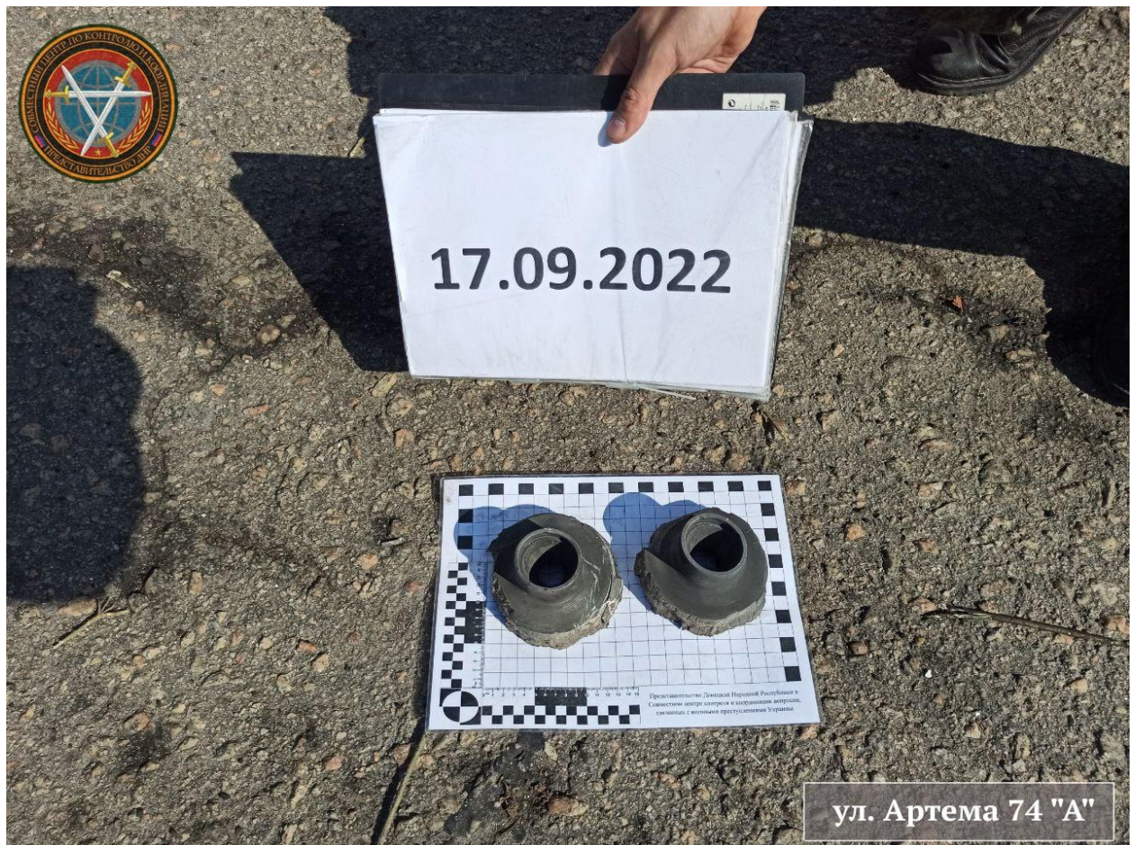
Fig. 13 – Nozzles of a NATO-standard M549 active-rocket projectile found by the JCCC representatives
