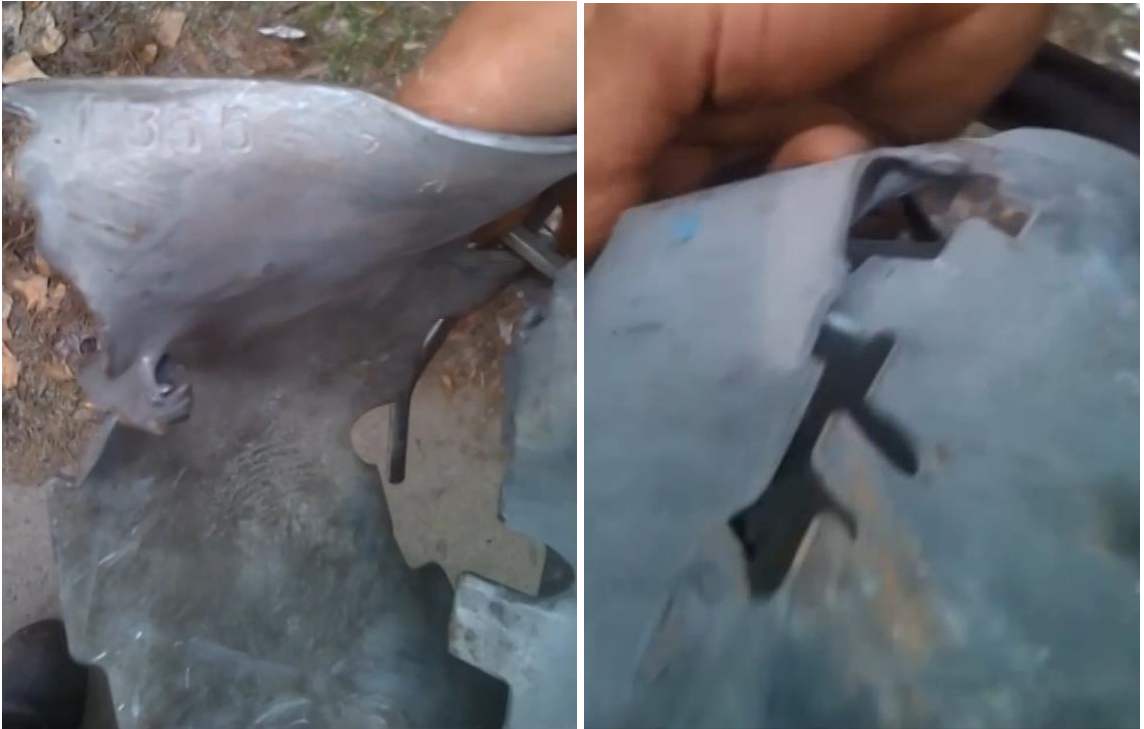
Fig. 27 - Remains of the rocket part of the 9K51 Grad MLRS projectile found at the site of shelling on 07.02.2015 in Kirovsk. The hole of the characteristic shape can be seen in the left figure; the hole of the characteristic shape, the rocket fin assembly and the embossed number “1355” are quite visible on the right. 45
