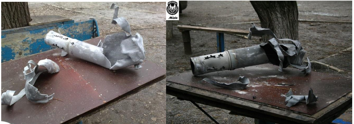
Fig. 26 - Remains of the rocket part of the 9K51 Grad MLRS projectile found at the site of shell hit 9 44 .
