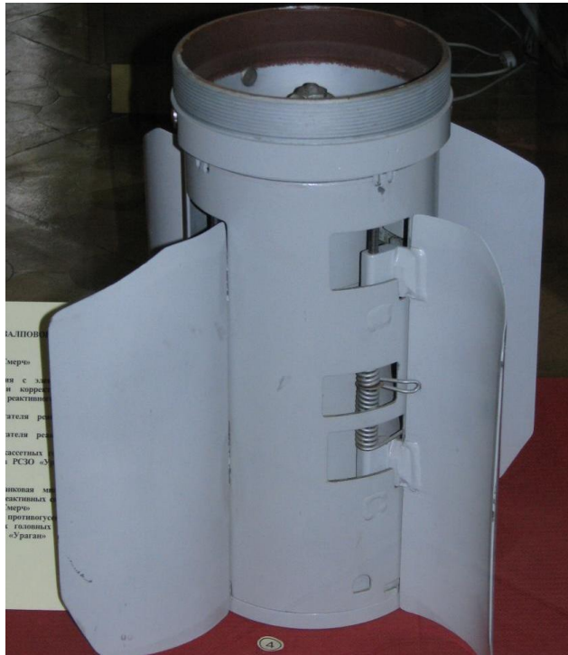
Fig. 30 – A dummy stabilizer control unit for the Uragan MLRS projectile 48 .
