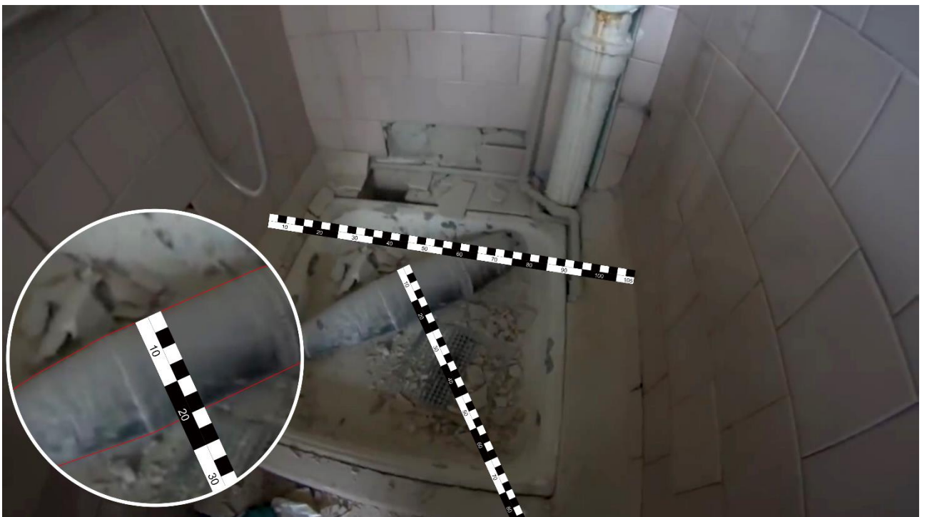
Fig. 18 – Measuring the projectile caliber using a scale ruler.
