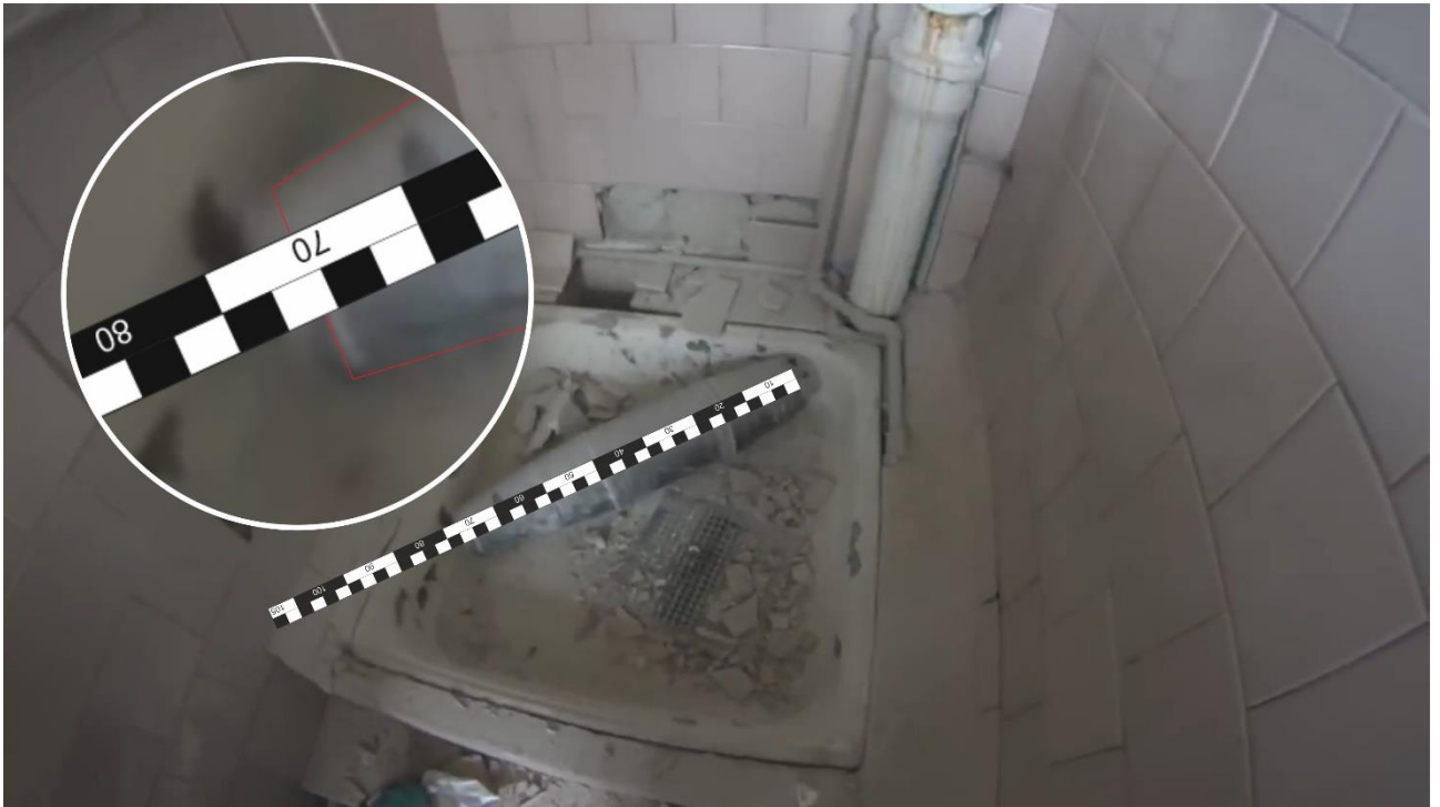
Fig. 19 – Measuring the length of the unexploded projectile using a scale ruler.
