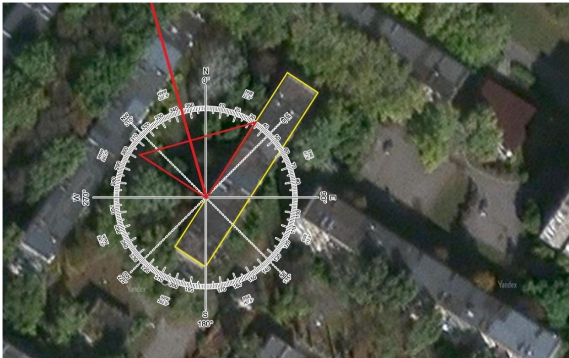
Fig. 22 – Fire direction determination using satellite imagery dated 16.07.2014 based on geometric constructions (shell hit 5).
