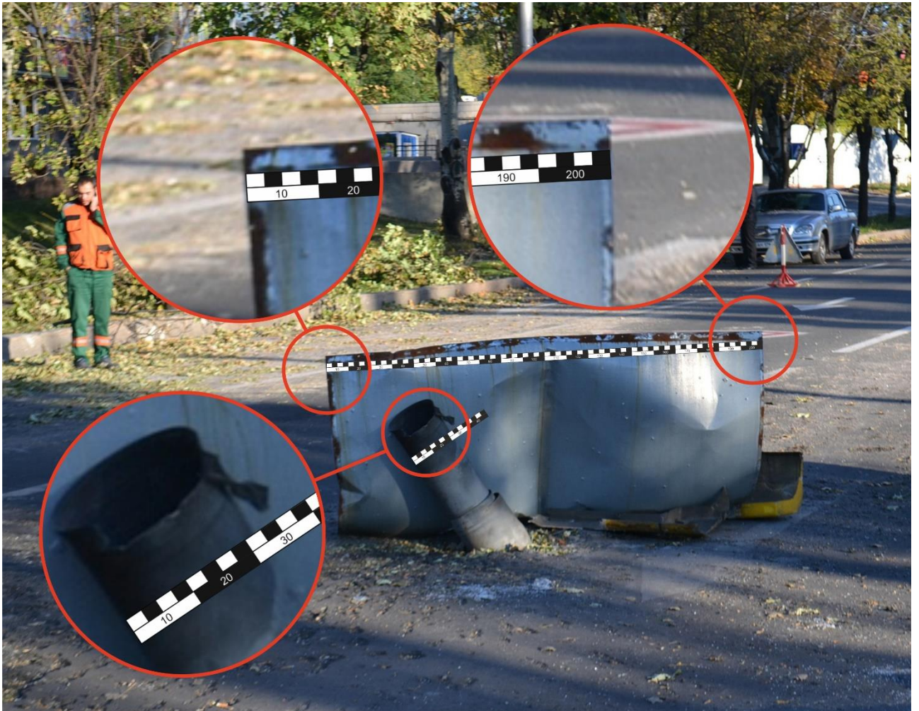
Fig. 4 – Measuring the projectile caliber using a scale ruler.
